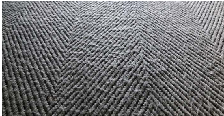
Pilling Example. Using the wrong vacuum will cause extreme pilling like this
